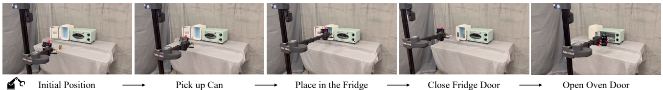
Fig. 6: Visualization of the trajectory VQ-BET generated in a long-horizon real world environment. Each demo consists of three to four consecutive tasks. Please refer to Table VI for the success rates for each task.
