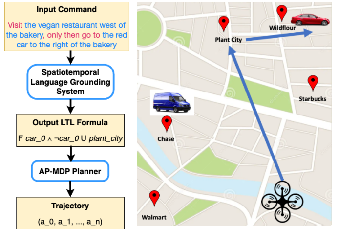
Fig. 2: An example shows an input spatiotemporal navigation command (the spatial and temporal elements are highlighted in blue and red, respectively), an output LTL formula whose propositions are grounded to physical landmarks, and an execution trajectory in the environment.
