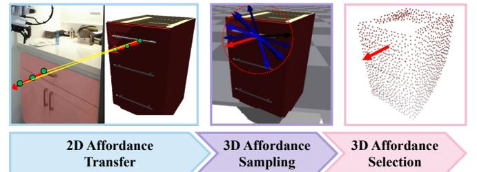
Fig. 4: Affordance transfer and lifting. Given a retrieved demonstration, RAM transfers the affordance in 2D via correspondence matching and obtains 3D affordance by sampling.
