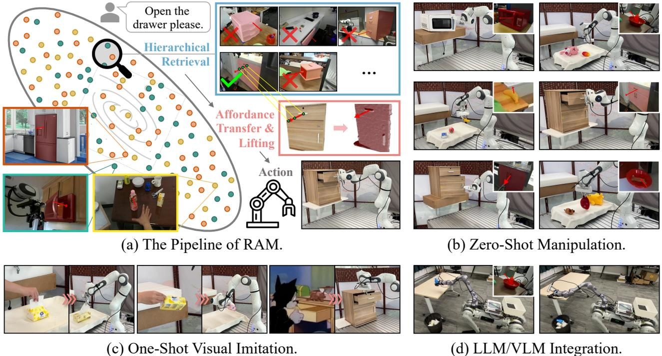
Fig. 1: (a) We extract unified affordance representation from in-the-wild multi-source demonstrations, including **robotic data**, **HOI data**, and **custom data**, to construct a large-scale affordance memory. Given language instructions, RAM hierarchically retrieves and transfers the 2D affordance from memory and lifts it to 3D for robotic manipulation. (b-d) Our framework shows robust generalizability across diverse objects and embodiments in various settings.
