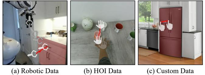
Fig. 2: Affordance annotation of demonstrations from various data sources. We extract unified affordance information automatically (for robotic and HOI data) or with minimal human effort (for custom data).
