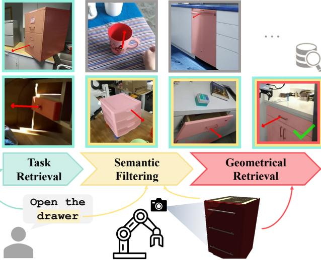
Fig. 3: Illustration of our hierarchical retrieval pipeline. RAM performs task retrieval, semantic filtering, and geometrical retrieval sequentially to retrieve the most similar demonstration from memory.
